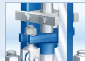
Gland packing / gland seal stuffing box provides an additional stem seal
